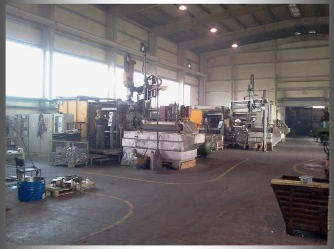
High Pressure Die Casting machines (7) : Buhler250t - Buhler 400t - Italpresse 550t - IDRA700t - TST Tebowa 800t - TST Tebowa 800t - IDRA950t
